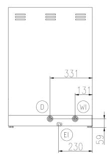
POWER CORD SUPPLY CABLE D'ALIMENTATION (EI) CABLE DE ALIMENTACION CANNA DI CARICO G 3/4 L=2000 mm G 3/4 INLET HOSE L=2000 mm TUYAU D'ALIMENTATION G 3/4" L=2000 mm TUBO DE ALIMENTACION G 3/4" L=2000 mm (WI)(D)
