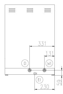
POWER CORD SUPPLY CABLE D'ALIMENTATION (EF) CABLE DE ALIMENTACION CANNA DI CARICO G 3/4 L=2000 mm G 3/4 INLET HOSE L=2000 mm TUYAU D'ALIMENTATION G 3/4" L=2000 mm TUBO DE ALIMENTACION G 3/4" L=2000 mm (WI)TUBO DI SCARICO Ø 29 mm L=2500 mm (D) DRAIN HOSE Ø 29 mm L=2500 mm TUYAU DE VIDANGE Ø 29 mm L=2500 mm TUBO DE DESAGUE Ø 29 mm L=2500 mm
